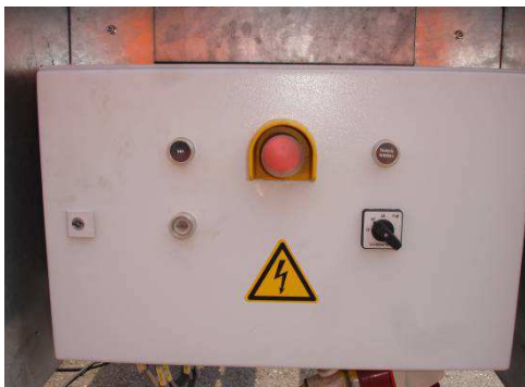
Figure 02 - Control console with Emergency Off switch
