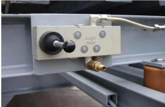
Figure 03: Manual valve - pneumatic system
